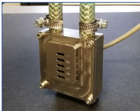
Figure 2.2 Custom-made GALAXI sample holder for five capillaries. The temperature control of the samples happens via the circulation of water in the back of the holder, allowed by the inlet and outlet.
